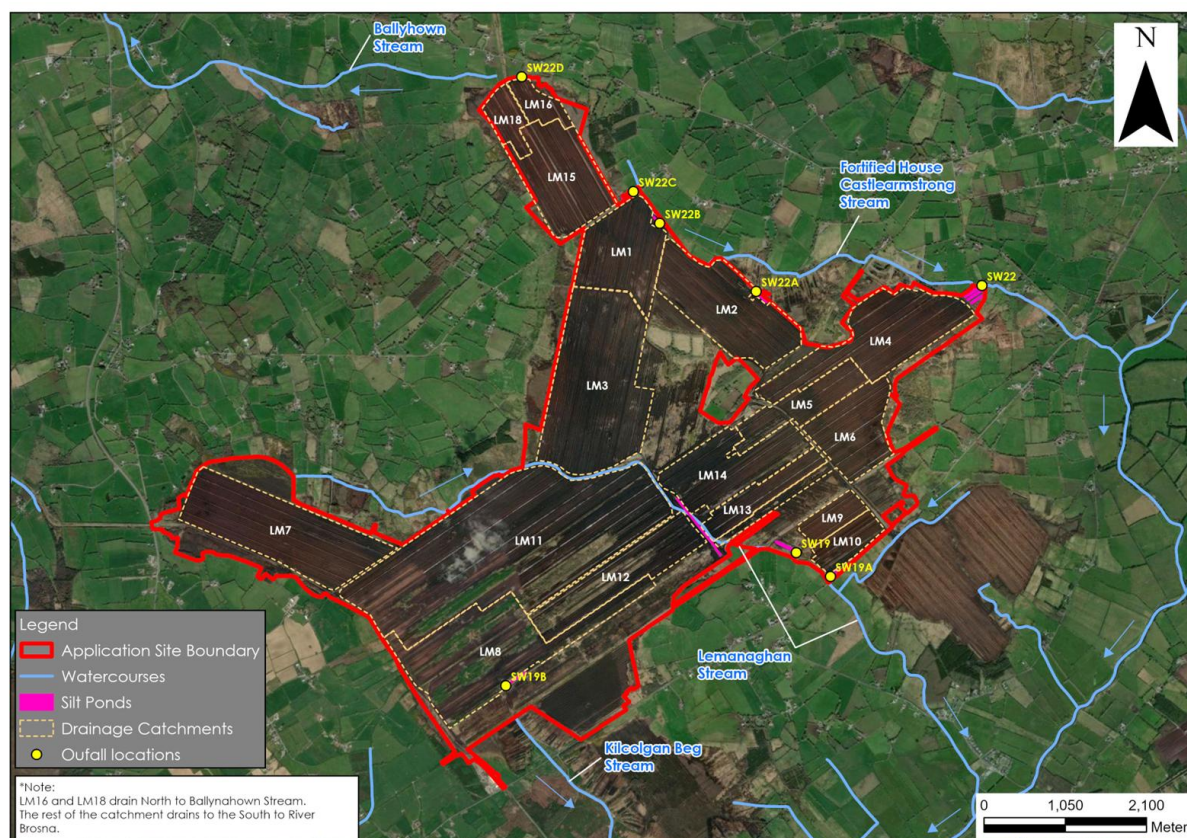
Figure B: Surface Water Outfall Locations
